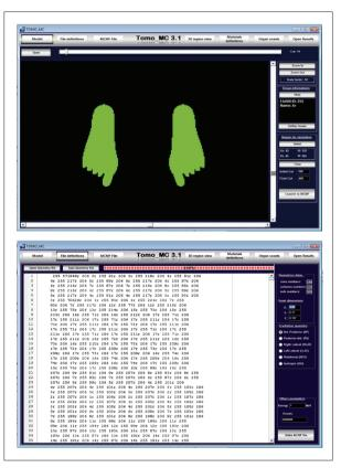
**Figure 2.** TOMO\_MC software for generation of MCNP input files from Voxels Models [18].
