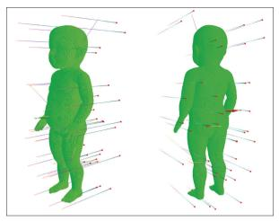
**Figure 4.** a) 3D visualization of the MCNP Input File geometry. b) Lateral view showing particle tracks resulting from the simulation of fifty 1MeV photons.
