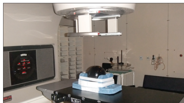
Figure 2. Experimental set up for FXG spherical phantom irradiation with 6 MV clinical photon beams using a Clinac 600C linear accelerator.
