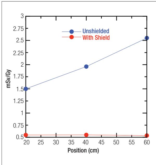
Figure 4. First configuration,  $H^*(10)_n$  at points along the X axis.
