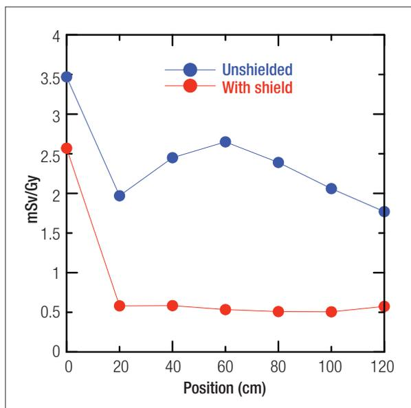
**Figure 3.** First configuration,  $H^*(10)_n$  at points along the Y axis.
