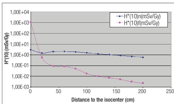
**Figure 1.** Comparison of the calculated values of ambient dose equivalent due to neutrons and photons, given in mSv for each dose in Gy deposited at the isocenter. (All for the Varian 2300 C/D).
