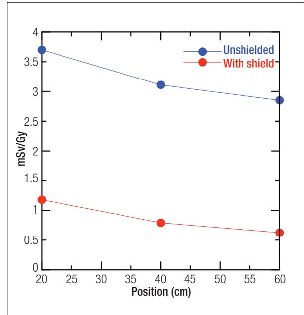
Figure 6. Second configuration,  $H^*(10)_n$  at points along the X axis.
