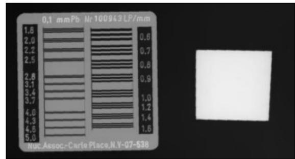
Figure 1. Radiograph: (a) the line-pair bar-pattern; (b) thick copper
