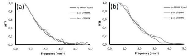
Figure 5. MTF obtained by (a) edge method and normalized at 0.6 lp/mm and (b) bar pattern.
