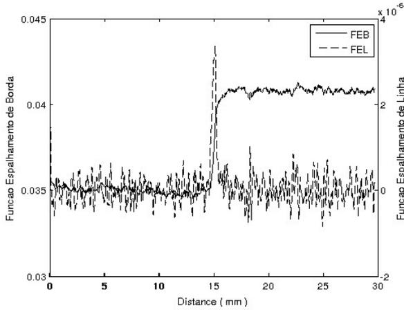
Figure 2. Real Supersampled Edge Spread Function (SESF) and line spread function (LSF) obtained from one of the radiographs used in this study.
