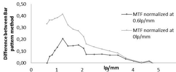
Figure 6. Difference between bar pattern and MTF normalized at 0 frequency and at 0.6 lp/mm.
