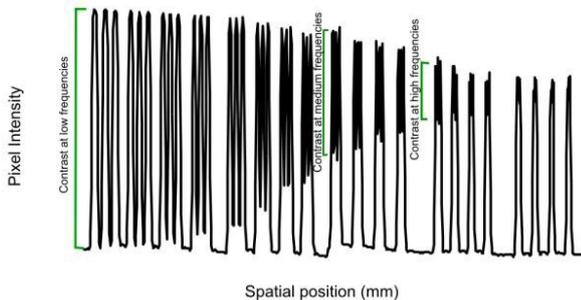
Figure 3. Contrast evaluation using the profile generated by the barpattern method.
