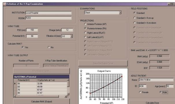
**Figure 2.** CALDose\_X user interface for the calculation of the INAK (ESAK), the selection of the X-ray examination and the definition of the patient data.
